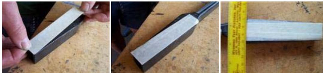
3) Take the tiller to the grinder, and grind away until you get to the line, making sure that you grind a flat surface away - not just round the bottom of your tiller!
